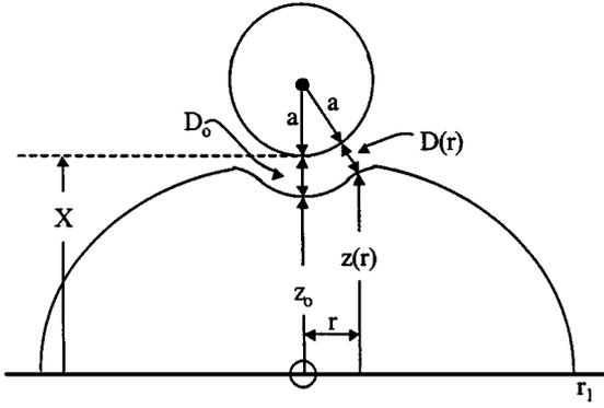
**FIG. A1.** The geometry of the probe/drop experiment. The drop has an undistorted radius of curvature,  $R_0$ , such that  $a \ll R_0 \ll \lambda$  so that gravitational distortion can be neglected. (The deformation is not shown to scale.)
