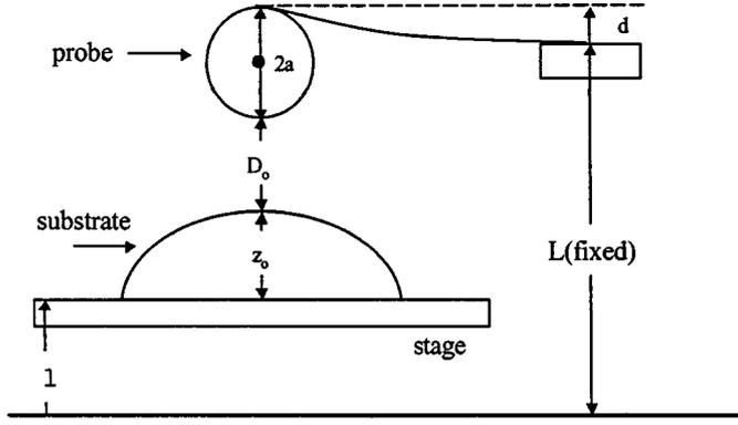
FIG. 1. Geometry of the AFM measurement.
