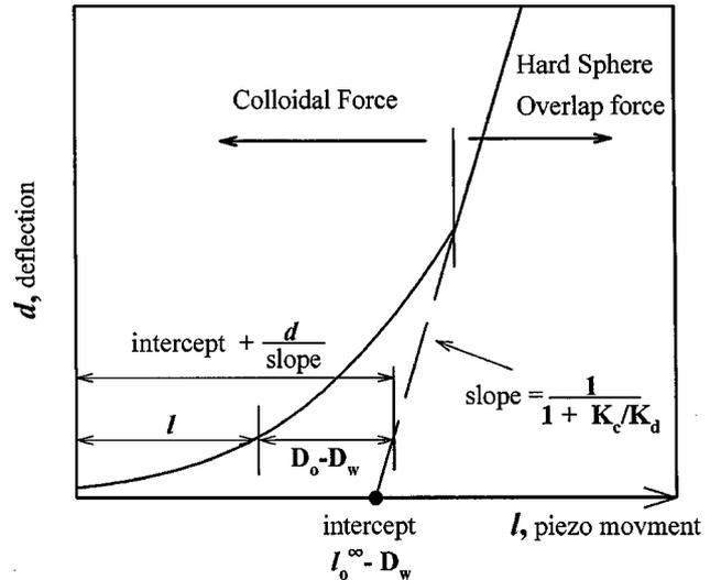
FIG. 2. The extraction of separation distance  $D_o$  from the linear compliance region.
