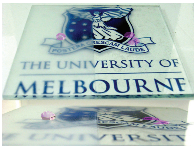
Fig. 1 Two views of the same glass plate where the slightly opaque half has been made into a silica nano-particle super-hydrophobic surface; the clear half is uncoated glass. The drops of water, tinted in pink, have a high contact angle on the super-hydrophobic side but spread on the uncoated side.
