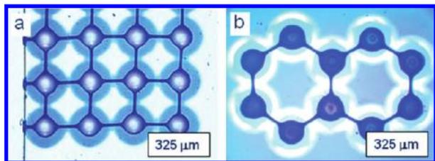
**Figure 4.** Micrograph views through the glass substrate showing (a) square and (b) honeycomb examples of liquid bridge networks formed using directly assembled  $250\ \mu\text{m}$  latex particle clusters with the respective geometry.
