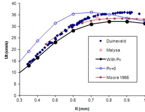
**Figure 1:** Terminal velocity of a rising 'clean' bubble as a function of the bubble radius  $R$ ; experimental data of Duineveld (1995) and Malysa et al. (2005) compared with the model with and without  $p_v$  term. Also indicated are the theoretical results of Moore (1965). The results with  $p_v$  slightly under-predict the experimental results of Duineveld (1995), and when  $p_v$  is neglected, they over-predict the terminal velocity for most radii.
