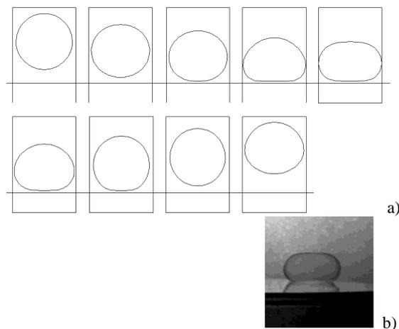
**Figure 4:** Soap bubble with initial radius 0.6 cm approaching a pool of stagnant water with 120 cm/s. a) Numerical results, time increases from left to right; compare 5<sup>th</sup> frame with image experimental frame. b) Experimental results (image reproduced from Vincent et al. 2007); only an image of the most deformed state is available for this experiment.
