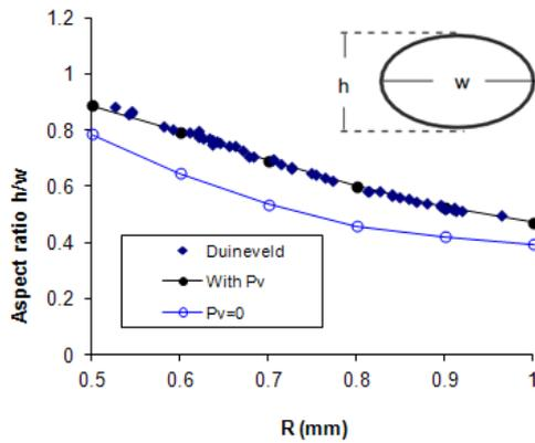
**Figure 2:** Aspect ratio (definition see inset) of the rising bubble for different bubble radii at terminal velocity. The results with  $p_v$  coincide with the experimental results of Duineveld (1995). When  $p_v$  is neglected, the model is clearly under-predicting the aspect ratio.
