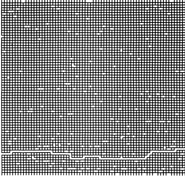
FIG. 4. An example of a simulation on a type-2(i) network with an exponential distribution of resistance values.
