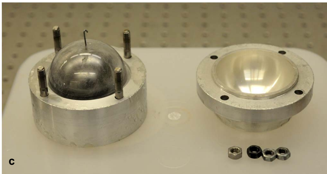
Supplemental Figure S1. (a) A schematic of the ice-shell-metal-core “ice(metal)” spheres prepared in an aluminium mold. (b) Photograph of the aluminium mold set inside the environmental chamber. (c) Photograph of the ice mold with the ice sphere inside shortly after removal of the mold top.
